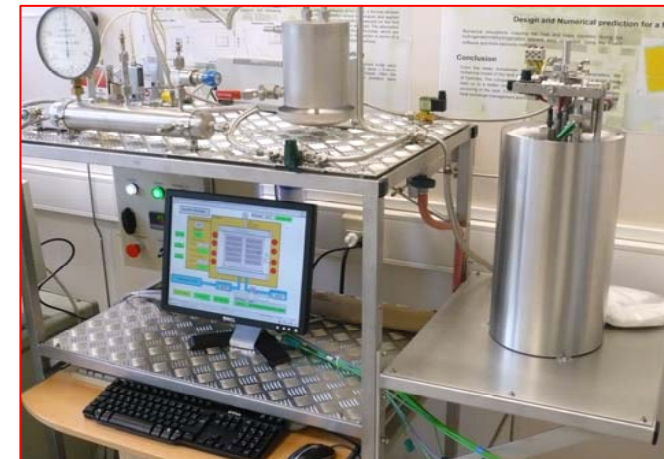
2 kg \text{MgH}_2 tank, \approx 5 kWh (120 gr - 1344 NL \text{H}_2 )
