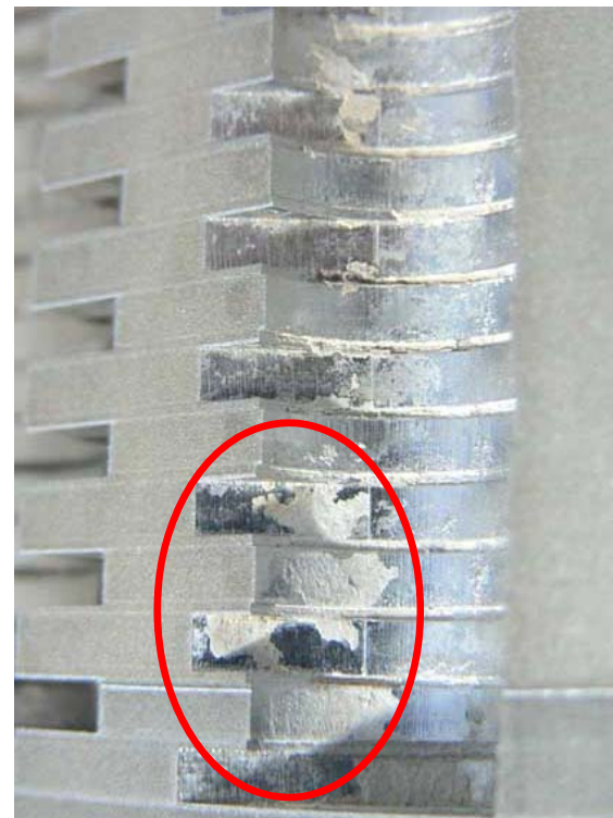
Plugged part inside heat exchanger
