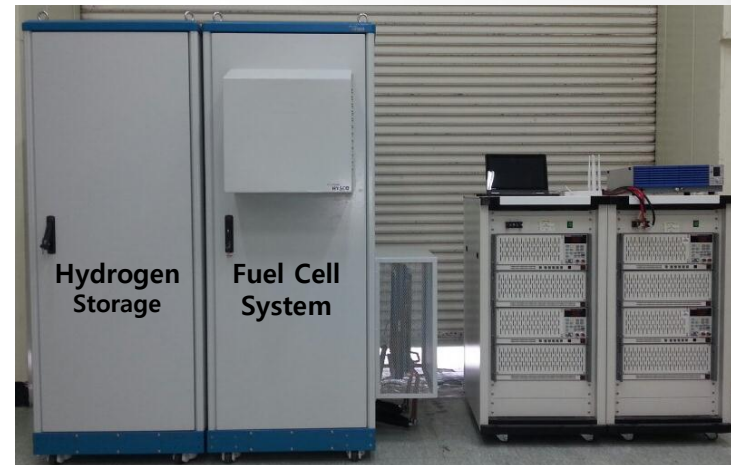
<2 Systems parallel test, with Cabinet>
