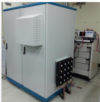
<2kW System with cabinet> ※ parallel available (4kW)
