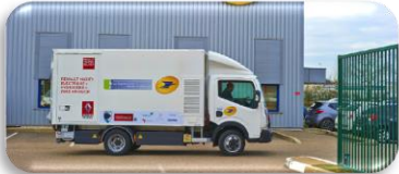
Renault Maxity Electric Truck with Fuel Cell Range Extender
